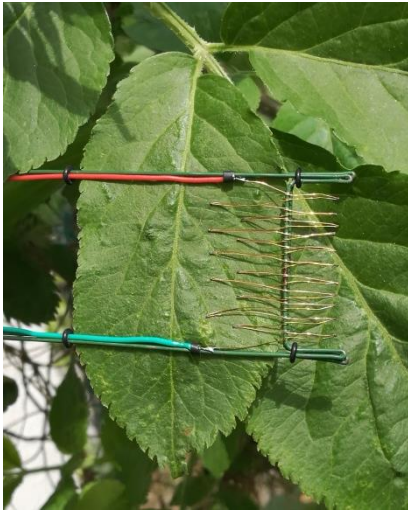
Type \Delta LA-B: Broad leaf version of the \Delta LA-Sensor ( \Delta T Leaf-to-Air)
