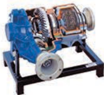
Viscous coupling differential Cutaway model
