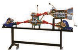
4x4 vehicle transmission assembly with 5 speed mechanical
