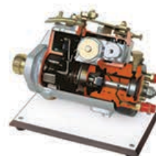
CAV DPC injection pump Cutaway model
