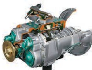
FULLER 13 SPEED GEARBOX cutaway model
