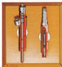
Diesel injector Cutaway model
