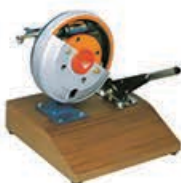
Drum brake Cutaway model
