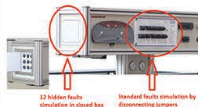
Hidden fault simulation for Engine control system
