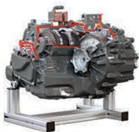
Direct shift gearbox Cutaway model
