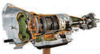
Automatic transmission Cutaway model
