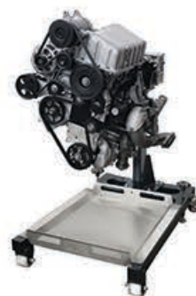
Turbo diesel engine with VE/ER pump for disassembling and assembling
