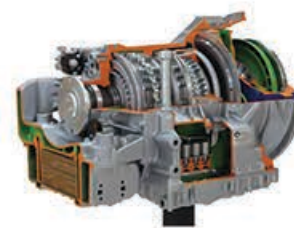
Heavy truck gearbox ZF 5hp Cutaway model
