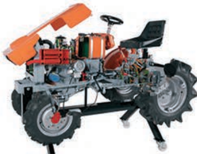
4 wheel drive farm tractor "KUBOTA" CUTAWAY MODEL
