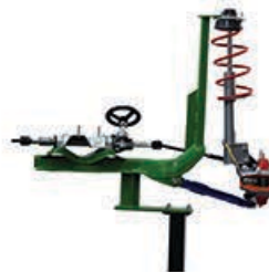
Sectioned front Suspension unit
