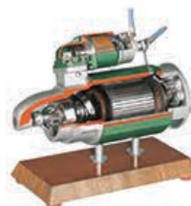
Starter motor with reduction gears Cutaway model
