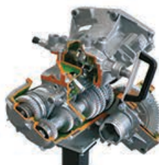
Gearbox front wheels drive Cutaway model
