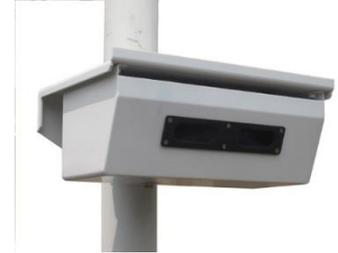
The visibility meter adopts light forward scattering principle, built-in microprocessor-controlled atmospheric visibility monitoring equipment. It emits pulses of infrared light and measures the intensity of the forward-scattered light of the suspended particles in the atmosphere, using suitable algorithms to convert the measurements to meteorological visibility values.
