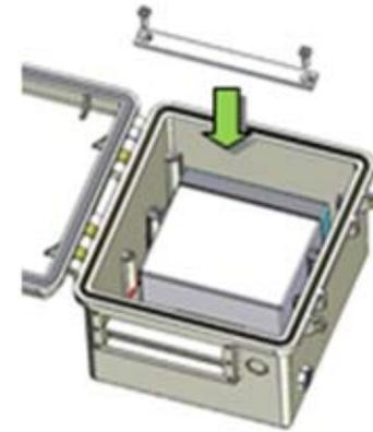
**CAUTION:** Make sure that battery cable is routed below the battery bar as shown to avoid possible shorting hazard!
