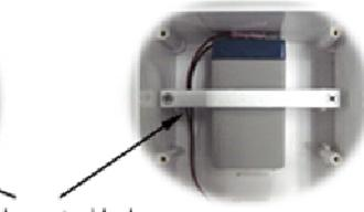
Cable routed below battery bar
