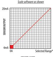
SENSED AMPS \*Factory calibrated ranges selected with the amperage range switch
