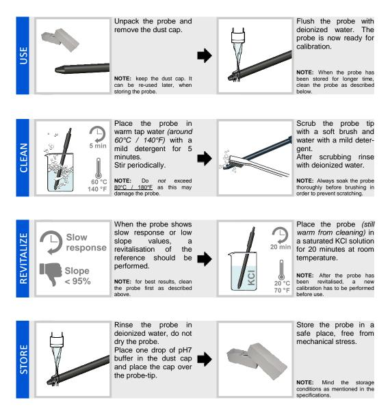
For accurate results always perform a calibration prior to use and periodically between measurements Visit www.specmeters.com for more information, full manuals and further product support.
