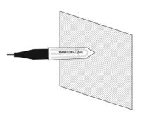
be taken to avoid snapping it during installation. To limit the effect of water moving vertically through the soil profile, the sensors should be installed so the flat face is perpendicular to the soil surface. For the same reason, if sensors are installed at multiple depths, they should be offset from one another.
