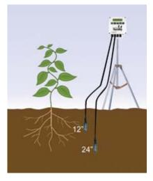
or two sensors should be installed in the root zone. A single sensor should be placed in the middle of the root zone. When two sensors are installed at a single site, it is recommended to place one sensor at the top of the root zone and a second at the bottom. An advantage of installing multiple sensors is it allows you to see how well irrigation and rainwater is moving through the soil profile.
