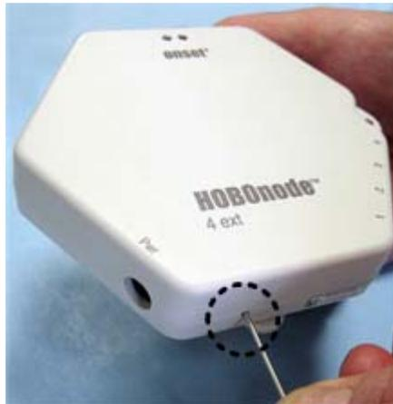
**LED Indication:** While the data node is searching for a receiver, the RED and GREEN LEDs will alternate blinking.
